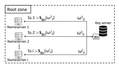
Figure 4.2: The delegation process in DNSSEC+: signing the nameserver short-term key structures by the long-term signing key of the zone.
