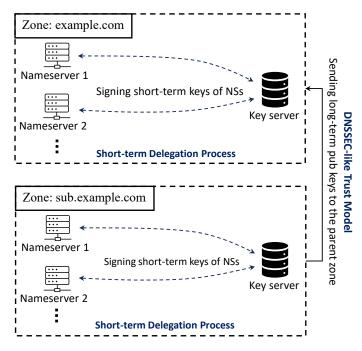
Figure 4.1: Zones in DNSSEC+ consist of a DNSSEC-like trust model (public key of each zone is authenticated by its parent zone) and short-term delegation.
