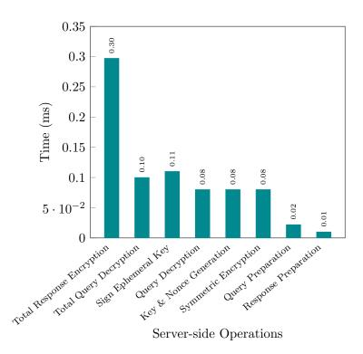
Figure 5.4: Breakdown of server-side processing latency for cryptographic operations
