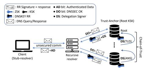
Figure 2.11: **DNSSEC:** Providing message authentication using digital signatures in Stage 2.
