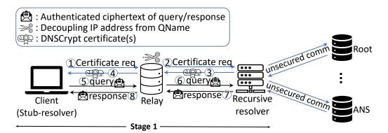
Figure 2.2: **DNSCrypt\*V3**: Using authenticated encryption in Stage 1, alongside the use of relay servers to enhance client privacy against resolvers.
