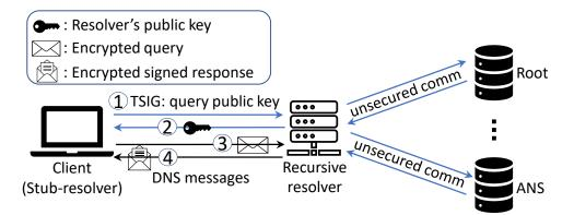
Figure 2.9: **CGA-TSIGe**: Enhancing name resolution by encrypting queries and encrypting and signing responses.
