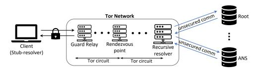
Figure 2.7: **DNS-over-Tor**: Based on Cloudflare's hidden resolver structure [144].
