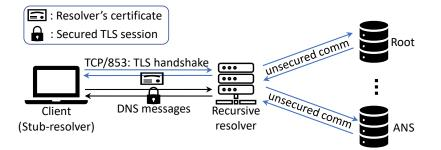
Figure 2.3: **DoT**: Sending DNS queries over TLS in Stage 1.
