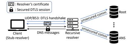
Figure 2.6: **DoDTLS**: Sending DNS over DTLS transport protocol.
