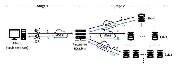
Figure 2.1: Complete DNS resolution process (divided into two stages): Prerecursive-resolver (Stage-1) and post-recursive-resolver (Stage-2).
