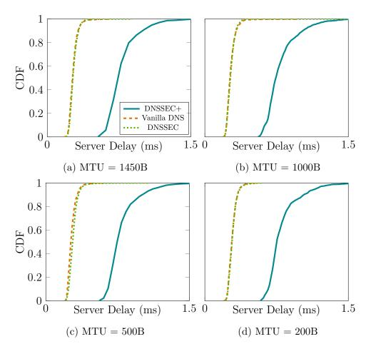
Figure 5.3: Server-side processing delay for DNSSEC+, Vanilla DNS, and DNSSEC in various MTUs.
