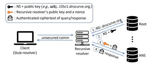
Figure 2.12: **DNSCurve**: Using authenticated encryption in Stage 2.
